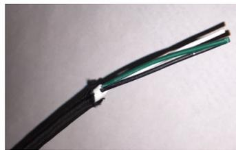
3) Bend Cord & remove outer Jacket, 3 conductor wires will be exposed. (White, Black & Green)
