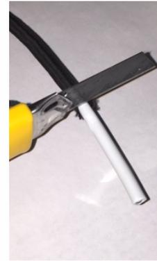
2) Mark 4" back around Cord ensuring to not cut inner wires.
