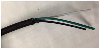
5) Use a Lighter to melt Outer Cloth cord .5" from inner Cord & remove. (**this only takes a second.**)
